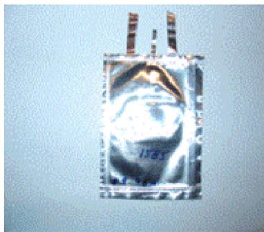
Figure 3: Photograph of the Li/C cell
