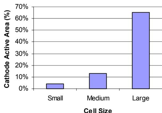
**Figure 6.** The cell case sizes with the percent of active area of the cathode.
