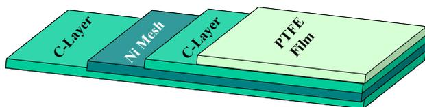
**Figure 1.** A diagram of the layered air cathode.
