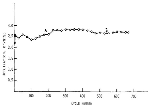
Figure 4: Cycle life data for a Na/NiS<sub>2</sub> cell (10)
