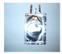
Figure 3: Photograph of the Li/C cell
